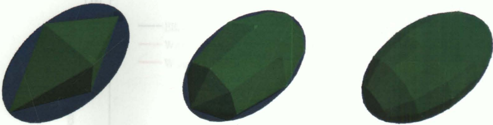
figure 25. Three polyhedron with different complexities approximating the same bounding ellipsoid. Using 6 vertices, 50 vertices and 170 vertices from left to right
